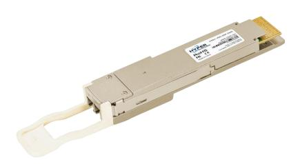
The 400G QSFP-DD ZR+ HO is a C-Band optical frequency tunable coherent optical module, combines 7nm coherent DSP ASIC functionality with best-in-class ultra-narrow line-width tunable lasers, high speed silicon photonics coherent modulators and high responsivity coherent receivers to deliver high performance at 100G DP-QPSK, 200G DP-QPSK, 300G DP-8QAM, and 400G DP-16QAM modulation formats. With integrated EDFA and VOA the TX output optical power is adjustable from -10dBm to +1dBm over the C-band.
